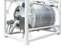
(Patent Pending) system controls the motor and slip clutches to maintain a constant tension on the umbilical whether the reel is full or near empty. The smart system also prevents the reel from deploying faster than the riser.
